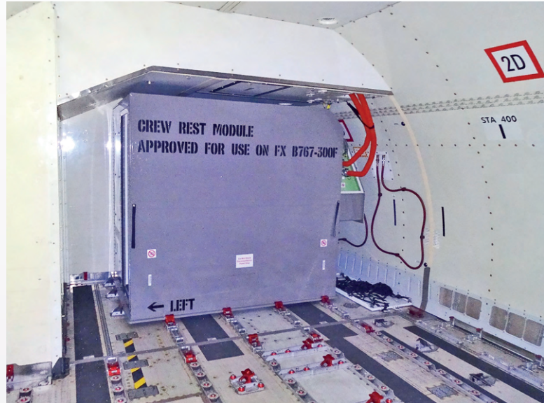
Installed Crew Rest Module
