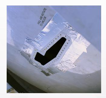
The EverLatch™ Cargo Door Latch by ATS is a cost-effective solution to a long-standing cargo door latch problem where operators experience fuselage skin and cargo door housing damage from sheared off nylon bumpers. The EverLatch is easy to install and is currently in service with airlines operating Boeing 737NGs.
