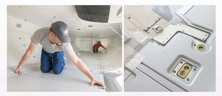
Through installation of the ATS CargoTek<sup>®</sup> Cargo Bay Protection Solution, unscheduled floor panel removals and secondary corrosion are eradicated. Airlines experience system-wide benefits resulting in greater operational efficiency and performance by avoiding cargo-related gate delays and related maintenance costs.
