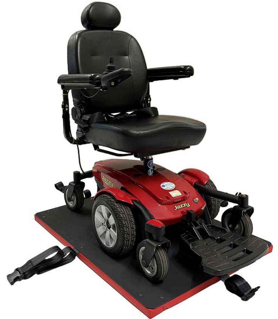
Power chair on PCCP prior to securing
