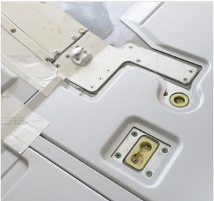
Cargo Tek® Cargo Bay Protection by ATS reduces cargo bay maintenance costs and cargo-related gate delays. Unprotected cargo bays are often damaged through routine use which can be avoided by installing ATS protection products.
