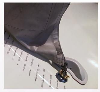
Cargo Tek® Net Anchor Guards by ATS prevent thrown or shifting cargo from damaging cargo net anchor fittings and sidewall liners. The guards are easy to install and are currently in service with airlines operating Boeing 737s.
