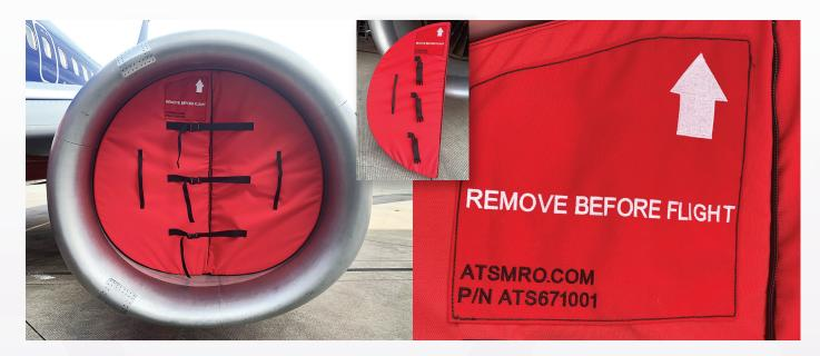
The FOD Protection Intake Plug by ATS is designed to protect the engine and engine components from damage due to debris and inclement weather. It is a cost-effective, easy to install solution for Boeing 737 NG aircraft.
