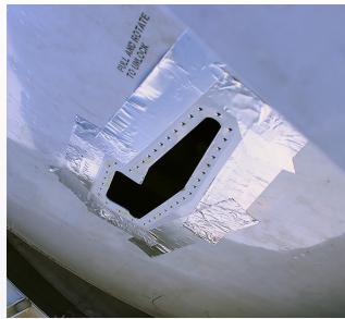
The EverLatch™ Cargo Door Latch by ATS is a cost-effective solution to a long-standing cargo door latch problem where operators experience fueselage skin and cargo door housing damage from sheered off nylon bumpers. The EverLatch is easy to install and is currently in service with airlines operating Boeing 737NGs.
